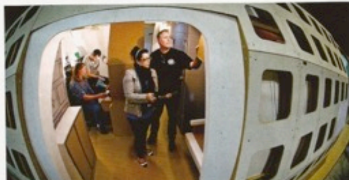
PHOTOS: (Left) Full-scale models at the Tanker Validation Center are used to help streamline the planned assembly process when KC-46A tanker production begins next summer. (Right) Looking up at the aft fuselage of a 767 commercial jetliner on the Everett, Wash., assembly line.
